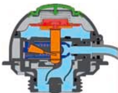
AutoMaXX® with positive pressure – valve open
